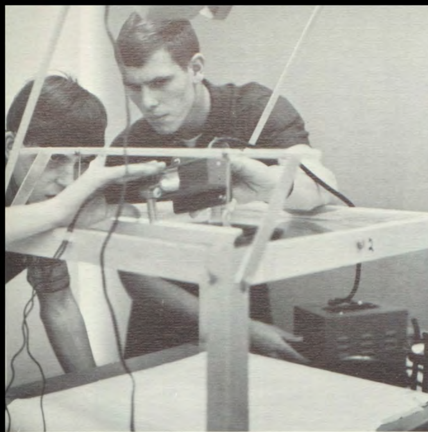
Using a thin layer of water to create waves, Bob Gossett and Roger Hart use a ripple tank to study light.
